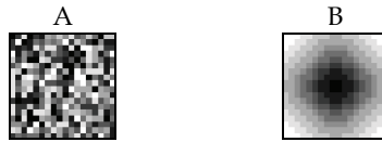
Fig. 2. Cost surfaces defined for multi-objective experiments: (A) uniform random and (B) conical (light color indicates higher costs if the location is occupied by patch cells).
